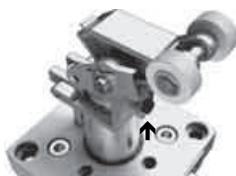
Sensing of the toggle lever position
