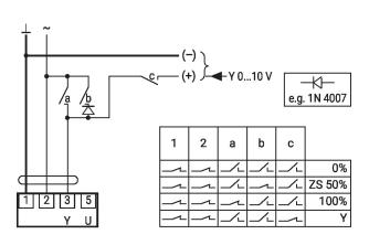
Override control with AC 24 V with Control remotely 0...100% with rotary switch positioner SG..
