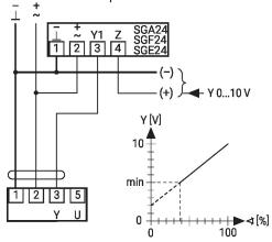
Control with 4...20 mA via external resistor
