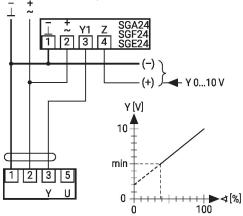
Override control with AC 24 V with Control remotely 0...100% with rotary switch positioner SG..
