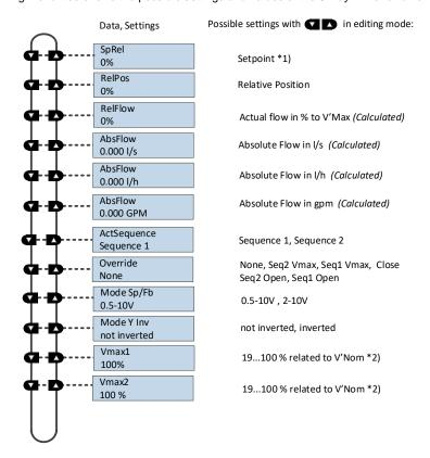
\*1) Setpoint for actuator between Vmax1 (Register No. 106) and Vmax2 (No. 107)
