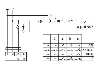
Override control with AC 24 V with Control remotely 0...100% with rotary switch positioner SG..
