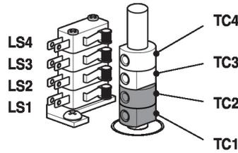
TC1/TC2 with sealing varnish: limit switches are secured against adjustment
