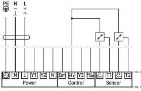
Switching contact connection (BACnet\_MS/TP / Modbus RTU)
