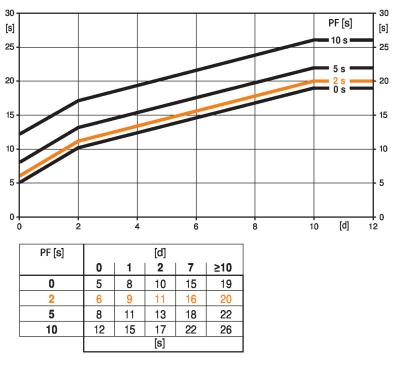
[d] = Electricity interruption in days [s] = Pre-charging time in seconds PF[s] = Bridging time Calculation example: Given an electricity interruption of 3 days and a bridging time (PF) set at 5 s, the actuator requires a precharging time of 14 s after the electricity has been reconnected (see graphic).
