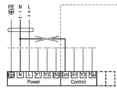
Power supply must not be connected to the signal terminals!
