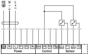
Switching contact connection (BACnet MS/TP / Modbus RTU)
