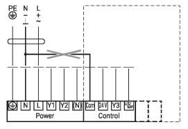
Power supply must not be connected to the signal terminals!
