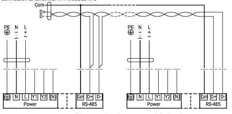
Connection BACnet MS/TP / Modbus RTU with analogue setpoint (hybrid mode)
