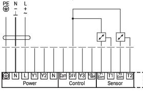
Switching contact connection (BACnet\_MS/TP / Modbus RTU)
