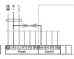
Power supply must not be connected to the signal terminals!
