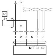
Switching contact requirements: The switching contact must be able to switch a current of 16 mA at 24 V accurately.
