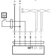
Switching contact requirements: The switching contact must be able to switch a current of 16 mA at 24 V accurately.
