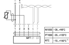
1) depending on type2) Resolution 1 OhmCompensation of the measured value is recommended
