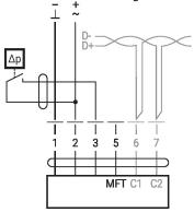
Switching contact requirements: The switching contact must be able to switch a current of 16 mA at 24 V accurately. Start point of the operating range must be parametrised on the MOD actuator as  $\geq 0.5 \text{ V}$ .
