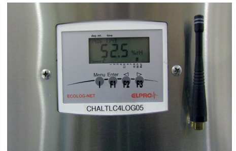
Temperature and humidity measurement with wireless link
