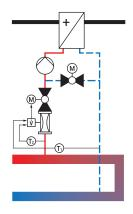
In general, one 3-way valve can be replaced by two 2-way valves. A DN 65...150 mixing circuit can thereby be realised with the products listed below.
