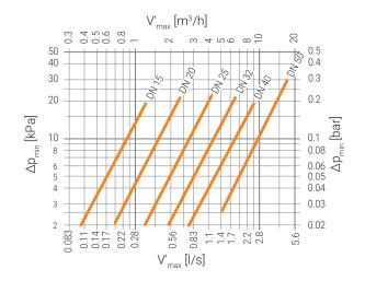
The 3-way Belimo Energy Valve is available in the nominal diameters DN 15...50. If a larger nominal diameter DN 65...150 is required, the following alternative can be considered.
