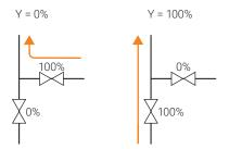
Control: both valves are operated with the same positioning signal. In order to represent the functionality of a 3-way valve, however, the actuator of the valve in the bypass is operated in an inverted manner.
