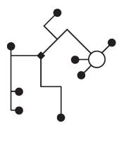
There are no restrictions for the network topology (star, ring, tree or mixed forms are permitted). Supply and communication in one and the same 3-wire cable • no shielding or twisting necessary • no terminating resistors
