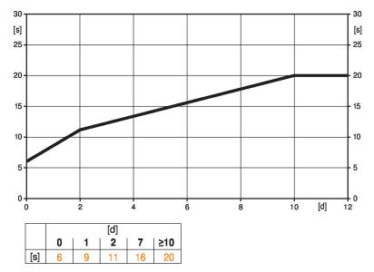
[d] = Power failure in days [s] = Pre-charging time in seconds
