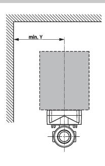
X/Y: Minimum distance with respect to the valve centre.
