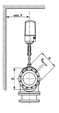
X/Y: Minimum distance with respect to the valve centre.
