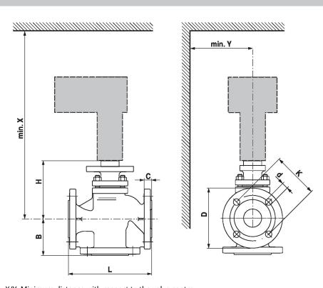
X/Y: Minimum distance with respect to the valve centre. The actuator dimensions can be found on the respective actuator data sheet.
