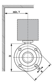
X/Y: Minimum distance with respect to the valve centre. The actuator dimensions can be found on the respective actuator data sheet.
