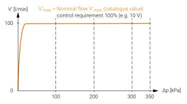
Pressure-independent flow over a large differential pressure range due to dynamic balancing (example EV032R2+BAC).
