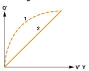
Depending on the design, temperature spread, fluid and hydronic circuit, the power Q' is not proportional to the water volumetric flow V' (curve 1). With the traditional type of temperature control, an attempt is made to maintain the positional signal Y proportional to the power Q' (curve 2). This is achieved by power control (see separate section).
