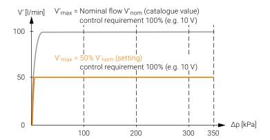
Plant-specific setting of the maximum flow V'<sub>max</sub> (Example: EV032R2+BAC)
