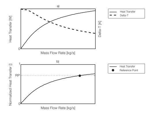
Figure 1: (a) Absolute and (b) normalized heat transfer capacity at design conditions. (The dip in the upper left corner of (a) is due to flow regime transition)
