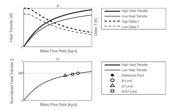
Figure 2: (a) Absolute and (b) normalized heat transfer capacity with flow, delta-T and flow/delta-T limiting results, assuming a 2K increase in chilled water supply temperature from 6 to 8°C.
