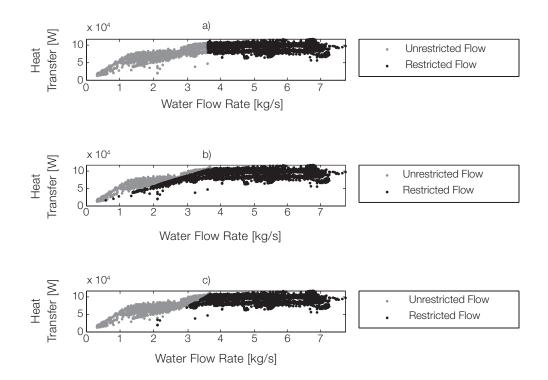
Figure 5: (a) Flow limiting (b) delta-T limiting and (c) flow/delta-T limiting coil management strategies applied to data from UCB air handling unit.
