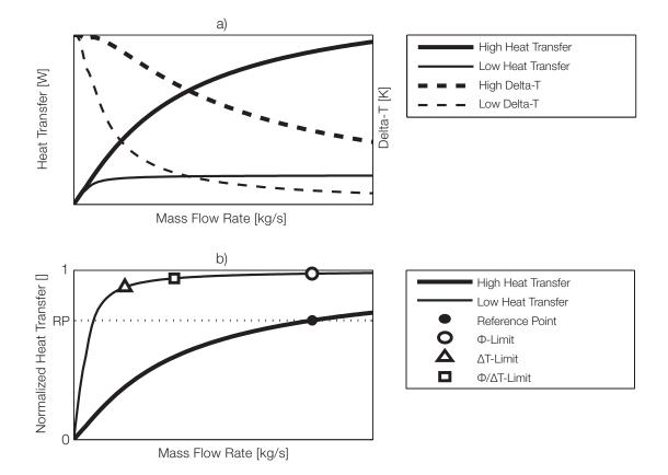
Figure 3: (a) Absolute and (b) normalized heat transfer capacity with flow, delta-T and flow/delta-T limiting results, assuming a factor 6 reduction in mass air flow rate.
