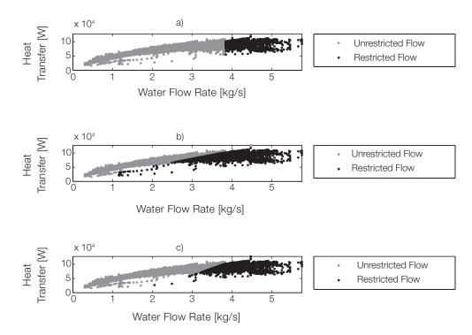
Figure 4: (a) Flow limiting (b) delta-T limiting and (c) flow/delta-T limiting coil management strategies applied to data from MIT air handling unit.
