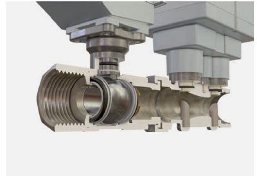
Abb. 14: Electronic PI valves have a simple flow path, which enables changes in the direction of flow to be dispensed with while at the same time significantly improving dirt tolerance.
