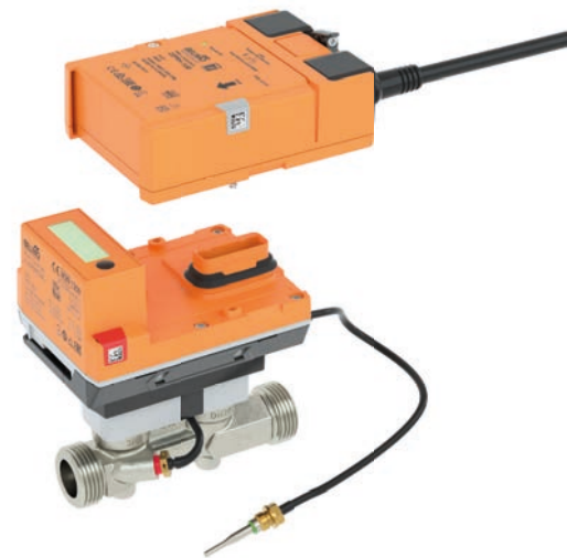
Abb. 40: All wiring is to the logic module, allowing the EN1434/MID sensor module to be recalibrated without disturbing the wiring.
