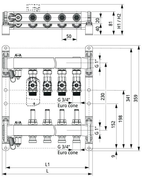
The actuator dimensions correspond to H1 (CQ.....A..) 105 mm and H2 (CQK...A..) 109 mm.
