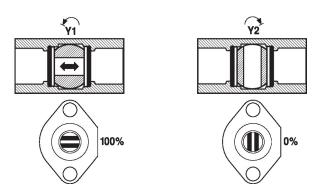
**Flow setting** The flow rate can be adjusted with the flow limiter between 0...5 l/min.
