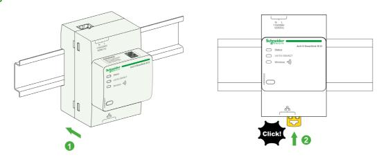
The following table describes the procedure for mounting the Acti 9 Smartlink SI D device on a DIN rail:
