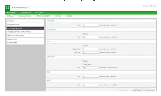
The Acti 9 Smartlink SI D supports HTTP/WEB, FTP, Modbus TCP, DNS, SNTP, and Discovery protocols and services. You can select the **Enable** check box and configure the port numbers for the **Modbus/TCP**, **FTP**, and **Discovery** protocols. If the discovery service is enabled, Acti 9 Smartlink SI D can be accessed from a laptop or a PC directly. The configuration of the network parameters is explained in detail in IP Network Services page (see page 71).
