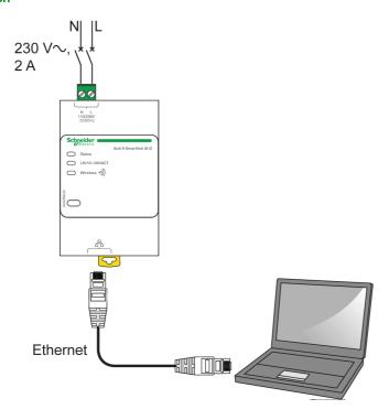
Acti 9 Smartlink SI D has an embedded web server. A web server is used to set Ethernet parameters or to display or control auxiliaries configured with Acti 9 Smart Test tool.
