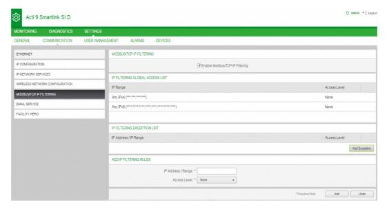
Follow the procedure to configure the IP address to enable write access:
