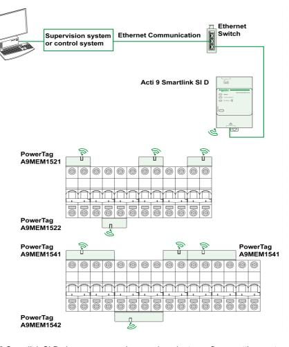
Acti 9 Smartlink SI D also manages web pages in order to configure settings or to monitor the wireless devices.
