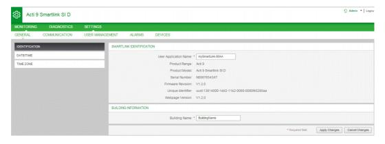
This page is used to read or modify the **User Application Name** that is used by the communication protocol to identify the device. For more details, refer the **Identification page** (see page 66) described in web page chapter.
