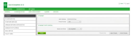
Follow the procedure to configure Ethernet parameters:
