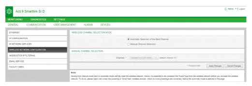
This page allows you to select the wireless channel either automatically or manually. Click **Automatic Selection of Best Channel** to select the channel automatically. Click **Manual Channel Selection** and select the channel from the available channels. The default channel is **Channel 11**.
