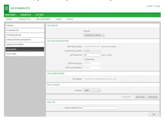
Click the **Enable** check box to configure the email server settings. Acti 9 Smartlink SI D allows you to select the **schneider-electric mail server** or **your own SMTP server** profiles from the drop-down list.
