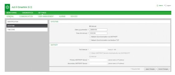
**NOTE:** After every power cycle, the device will reset to a default value of date and time. The default date and time value is 2000/1/1, 00:00:00.
