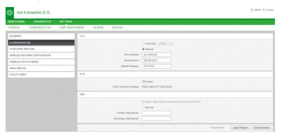
IPv4 parameters can be set either in manual mode or in automatic mode. To configure IPv4 parameter in automatic mode, click **Automatic** and select the type of protocol (DHCP or BOOTP) from the list. The default type is **DHCP** protocol.
