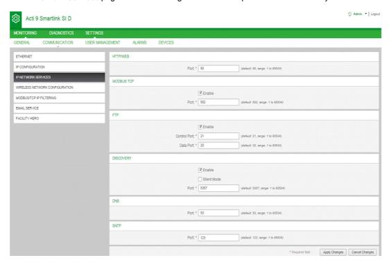
The Acti 9 Smartlink SI D supports HTTP, Modbus/TCP, FTP protocols, DNS, SNTP, and discovery services.
