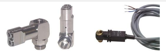
This pneumatic sensor is used to detect the end position of a cylinder. It works by measuring the pressure drop at the outlet chamber of the cylinder when it reaches the end of the stroke. Pneumatic sensor fittings replace limit switches. The sensor is screwed into the pneumatic ports of the cylinder. It scans the working pressure of a cylinder by screwing into its input hole. The screw connection switches from (P) 1 to (S) 5 when there is no pressure on the screw connection.
