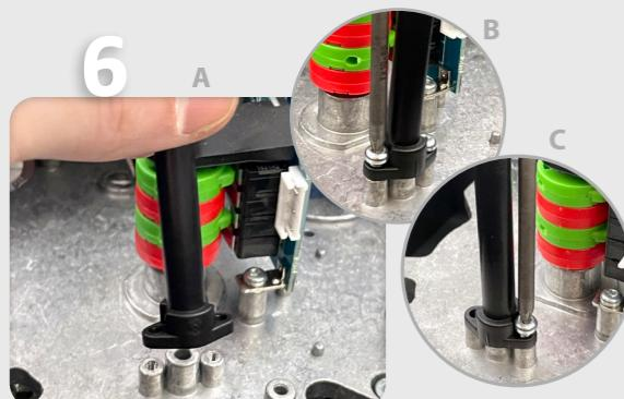
Fix the plastic column (Element B) on the base plate, by using 2 sheet metal fixing screws (Element D) (Fig. A,B and C).
