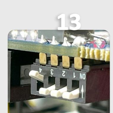
Use the configuration you need by moving the DIPs, according to the instrumentation signal:
