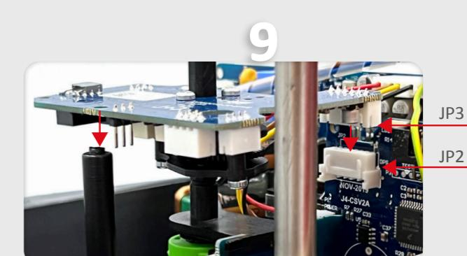
Press the DPS positioner PCB (Element C) along the shaft until the PCB connector (JP3) is plugged in the actuator PCB connector (JP2).
