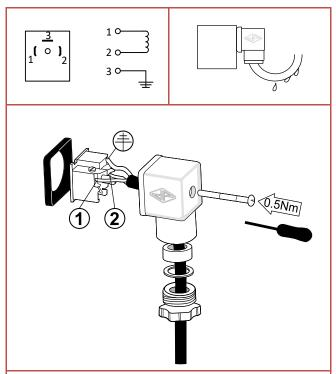
Connector: EN 175301-803 Type A (formerly DIN 43650A).
