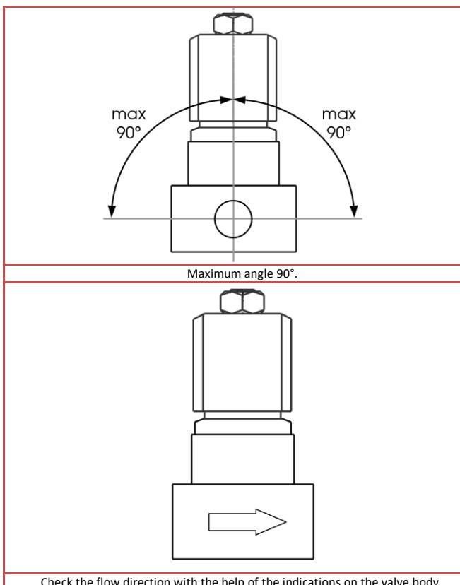
Check the flow direction with the help of the indications on the valve body.
