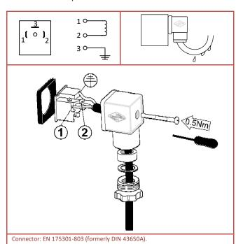
The poles (1) and (2) should be connected to the power supply, polarity is not important. Pole (3) is the ground. Connect the connector thoroughly to avoid ingress of moisture. Ensure that drops cannot slip along the cable and enter the connector
