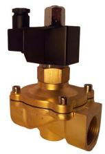
The DF-SB is a semi-direct operated 2/2-way solenoid valve. The valve is normally open. The solenoid valves have an orifice of 16 to 25 mm, operate from 0 bar and are suitable for medium flow rates. The body is made of brass or stainless steel with NBR, EPDM or FKM seal. The DF-SB solenoid valves are compatible with all coils from the CS2-series.
