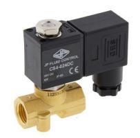
The CM-DA is a direct operated 2/2-way solenoid valve, specially designed for installations where compactness and energy efficiency is important. The valve is normally closed. The solenoid valves have an orifice of 1 to 2.5 mm, operate from 0 bar and are suitable for small flow rates. The body material is made of brass or stainless steel with a NBR, EPDM or FKM seal. The CM-DA solenoid valves are compatible with all coils from the CS4 series.
