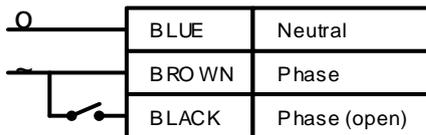
Connecting the control wire (black) opens the valve in 16s. Once the control wire shuts down, the valve closes in 16s. The actuator consumes energy only during opening and closing.
