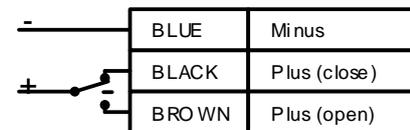
Connecting the brown control wire, the valve closes in 6s. Connecting the black control wire, the valve opens in 6s. If both control wires are connected, the position of the valve can be regulated. **Never connect the black and brown control wires at the same time!** This will damage the actuator. The actuator consumes energy only during opening and closing.
