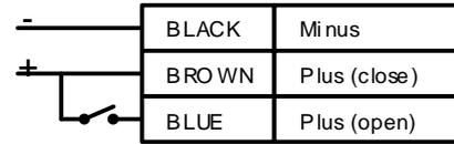
Connecting the control wire (blue) opens the valve in 6s. Once the control wire shuts down, the valve closes in 6s. The actuator consumes energy only during opening and closing.
