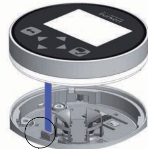
The display module or the Wi-Fi module is unlocked
