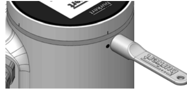
The blind cover or the display module or the Wi-Fi module is locked
