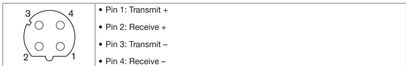
Fig. 36: Pin assignment of the 4-pin M12 female connector
