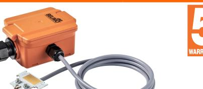
For detection of condensation on chilled surfaces (e.g. chilled beams). With relay contact for connection to controller and display systems or for series connection with the cooling valve to interrupt the cold water flow directly when condensation begins.
