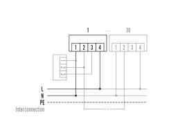
230-V connection. Also available networking with max. 30 detectors (max. line length 300 m) and PROTECTOR K relay.
