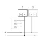
9-V battery operation. Optional networking with max. 30 detectors (max. line length 300 m) and PROTECTOR K relay.
