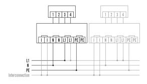
Standard operation. Also available Networking with max. 30 detectors (max. line length 300 m). Filter to prevent network interference on the PROTECTOR K 230 V.
