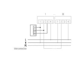
$230 \hbox{-V connection. External switching relay for switching external devices such as sirens, flash lights and telephone diallers.}$
