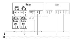
Standard operation with optional control via a closing button and use of max. ten slave devices to one master device.
