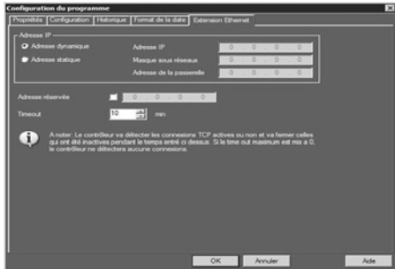
Ethernet extension configuration window
