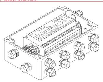
The Remote Monitoring Modules (RMM2) provide temperature monitoring capability for nVent RAYCHEM NGC controller family. The RMM2 accepts inputs from up to eight Pt 100 temperature sensors that measure pipe or ambient temperatures in a heat-tracing system. Multiple RMM2 units communicate with a single nVent RAYCHEM NGC User Interface Terminal (nVent RAYCHEM NGC-UIT) providing centralised monitoring of temperatures.
