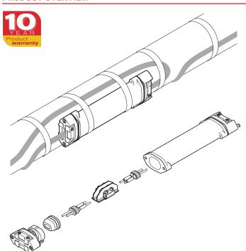
The nVent RAYCHEM S-150 is a cold applied low profile splice for in-line connection. This universal kit fits with all nVent RAYCHEM industrial heating cables, BTV, QTVR and XTVR, meaning simplified product selection and reduced inventory to stock. It can be used in applications with temperatures ranging from  $-55^{\circ}\text{C}$  to 200°C. It is approved for use in hazardous areas.
