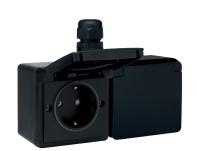
points of this double, horizontal box are situated 50 mm apart on a vertical axis and 71 mm apart on a horizontal axis. This size indication is indelibly imprinted on the bottom of each box. The oval screw openings allow for imprecise drilling. By forming a pressure lock, a gasket ensures the protection degree and the double insulation. The box contains two diagonal, knock-out condensation openings.
