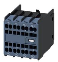
Auxiliary switch on the front, 2 NO + 2 NC Current path 1 NC, 1 NC, 1 NO, 1 NO for 3RH and 3RT spring-type terminal .1/.2, .1/.2, .3/.4, .3/.4
