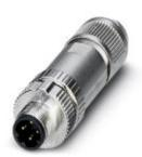
Connector, PROFINET CAT5 (100 Mbps), 4-position, shielded, Plug straight M12, D-coded, Push-in connection, knurl material: Zinc die-cast, nickel-plated, external cable diameter 4 mm ... 8 mm
