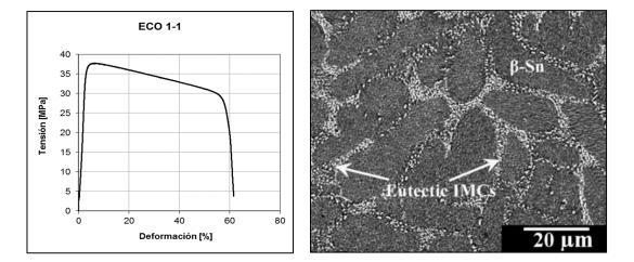
Figure 1. a)Stress-Strain curve and b)SEM image for ECO 1 solder.
